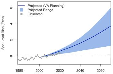
The graph shows the projected change of sea level in feet above NAVD88 compared to the 1983-2001 average. The blue line shows the sea level rise scenario used for official planning purposes in Virginia. The blue shading shows the range between the low and extreme scenarios for sea level rise. Dots show the observed changes in sea level at Sewell's Point, VA. Data for the future scenarios are retrieved from the National Oceanic and Atmospheric Administration (NOAA).
